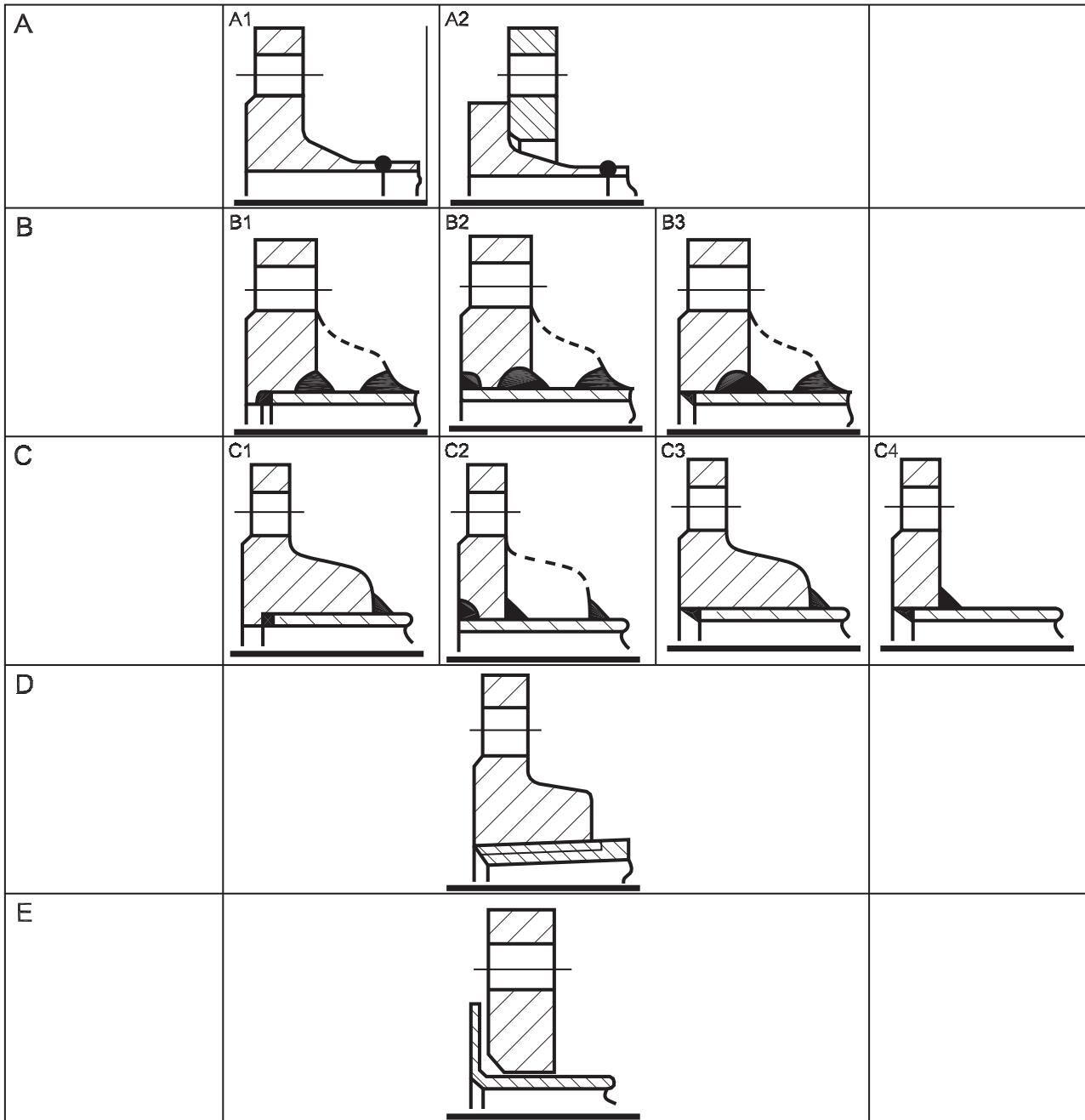
Figure 1 : Types of metallic flange connections
