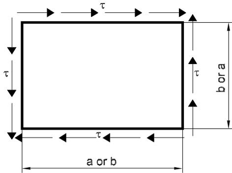
**Figure 4 : Buckling of a simply supported rectangular plate panel subjected to bi-axial compression and shear (1/1/2017)**
