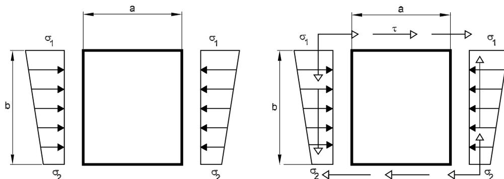
**Figure 3 : Buckling of a simply supported rectangular plate panel subjected to shear**
