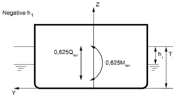
Figure 2 : Wave loads in load case “b”
