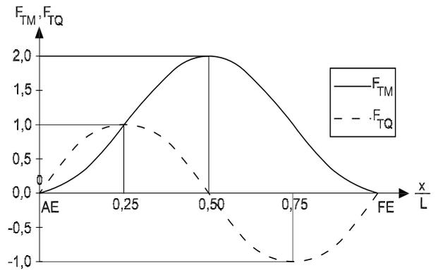
**Figure 6 : Ship condition 2 - Distribution factors  $F_{TM}$  and  $F_{TQ}$**
