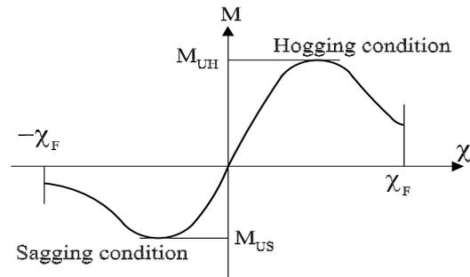
Each step of the incremental procedure is represented by the calculation of the bending moment  $M_i$  which acts on the hull transverse section as the effect of an imposed curvature  $\chi_i$ .
