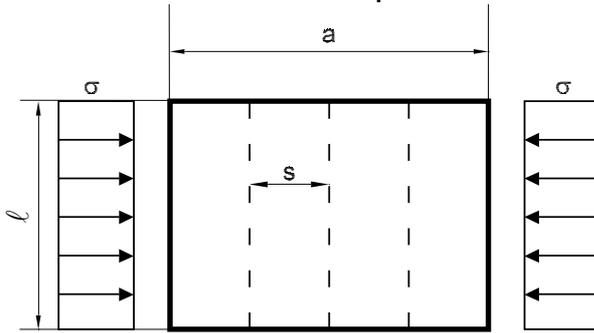
Where intercostal stiffeners are fitted, as shown in Fig 7, the check of the moment of inertia of stiffeners perpendicular to the direction of compression is to be carried out with the equivalent net thickness  $t_{eq,net}$ , in mm, obtained from the following formula:
