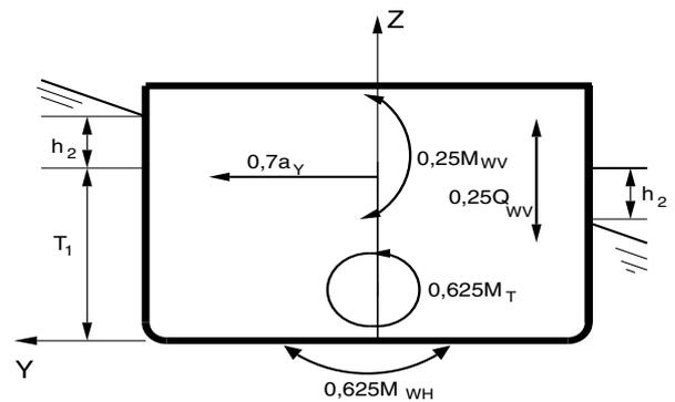
Figure 4 : Wave loads in load case “d”
