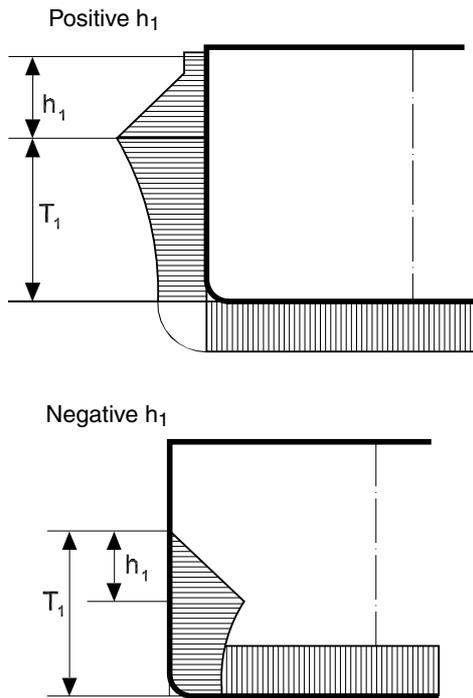
Figure 3 : Wave pressure in load case “b”
