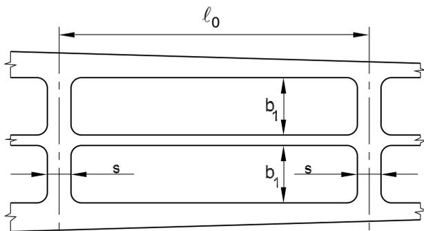
**2.1.5 Longitudinal bulkheads with vertical corrugations**
