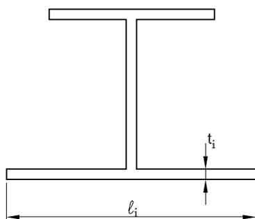
Figure 4 : Beams of double skin structures
