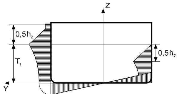
**Table 3 : Wave pressure on sides and bottom in upright ship conditions (load cases “a” and “b”)**
