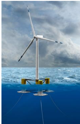
Figure 1: Floating Offshore Wind Turbine Installation (semi-sub)
