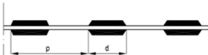
Figure 1 : Intermittent chain welding (1/7/2025)
