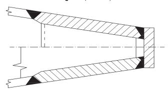
The plate thickness of a shaped plate stem and, in the case of a blunt bow, any part of the shell which forms an angle of 30° or more to the centreline in a horizontal plane, is to be not less than 1,3 times the thickness of the adjacent shell plating calculated according to [6].
