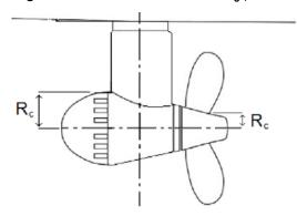
For impacts on non-hemispherical areas, such as the impact on the nozzle, the equivalent impact sphere radius is to be estimated using the equation below.
