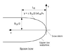
Figure 5: Example of  $e_b$  effect on the bow shape for  $B_{III} = 20$  and  $L_B = 16 (1/1/2021)$
