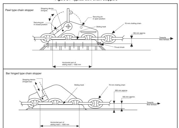
Figure 2: Typical bow chain stoppers
