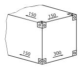
Figure 13: Permissible transverse and vertical compressions on frames of 20' and 40' containers
