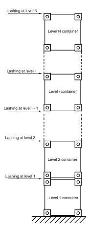
**4.3.3** Where empty containers are stowed at the top of a stack, the still water and inertial forces are to be calculated considering mass of empty container equal to:
