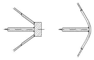
The plate thickness of a shaped plate stem and, in the case of a blunt bow, any part of the shell where  $\alpha \geq 30^\circ$  and  $\psi \geq 75^\circ$  ( $\alpha$  and  $\psi$  defined in Sec 1, [3.1.1], is to be not less than that calculated in [5.1.2] assuming that:
