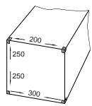
**6.2.2** In case of a combination of forces applied on container corners, the resultant force is to be less than the value obtained, in kN, from Fig 16.
