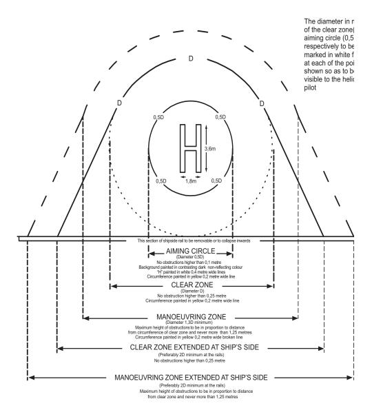
Figure 1: Landing area at the ship's side (1/7/2010)
