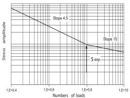
Figure 8 : Constant-slope S-N curve (1/1/2010)
