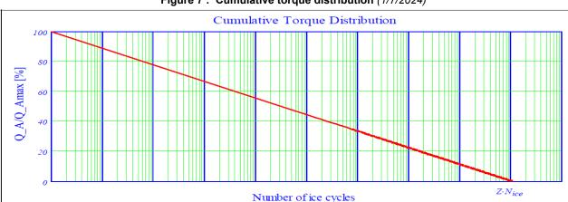
Figure 7: Cumulative torque distribution (1/7/2024)
