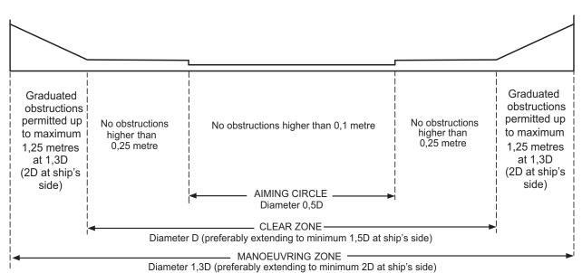
Figure 3: Landing area - permitted height of obstructions (elevation) (1/7/2010)
