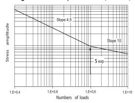
Figure 6: Constant-slope S-N curve (1/7/2024)
