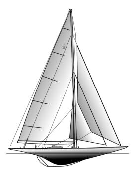
BOOM - Horizontal spar, attached to the Mast, designed to controling, supporting, containg the sail.
