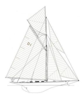
HALYARD(s) - They are line(s) (ropes) used to hoist or raise sails and other rigging elements, such as flags or spinnaker poles, up the mast. Halyards typically run from their attachment points on the sail or rigging element to the masthead or other designated hoisting points on the mast.
