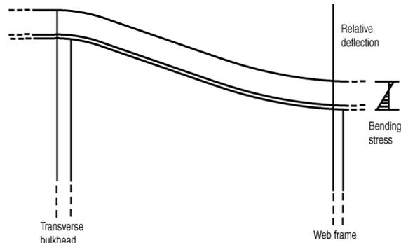
**Figure 2: Types of stresses for the fatigue analyses**
