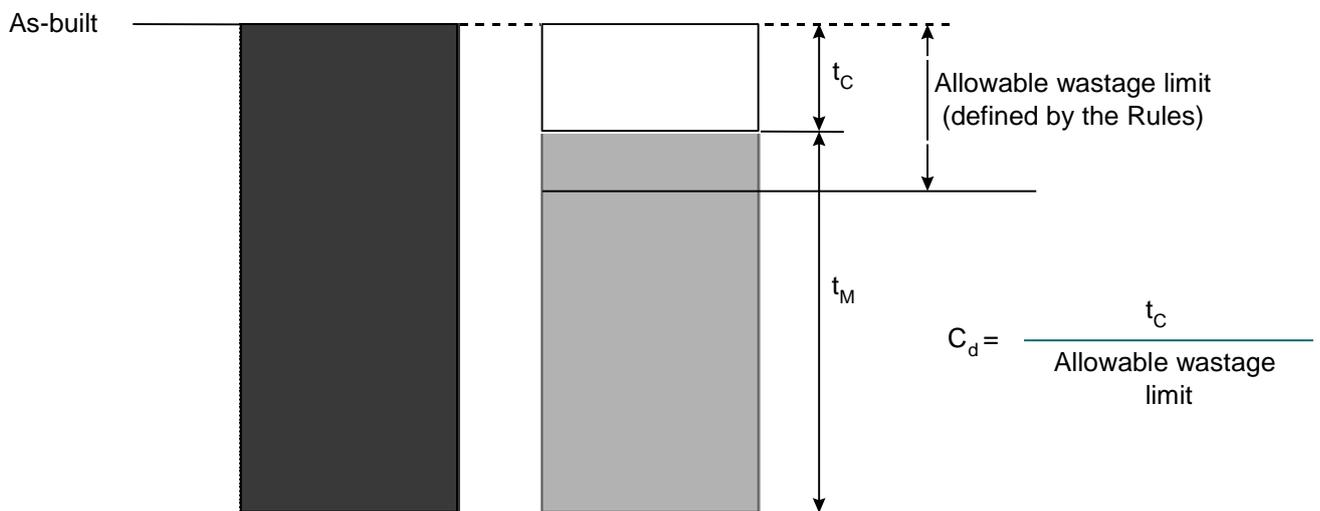
$t_c$  is the thickness diminution due to corrosion
