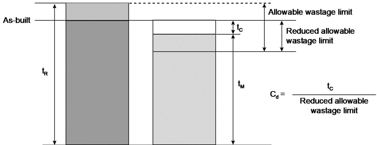
Figure 5b: Corrosion diminution  $C_d$  in the case  $t_R < \text{As-built}$
